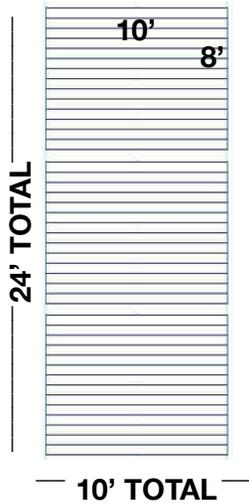
With a smaller stabilized entry of 10' wide, only one 8' X 10' **TOG or TOP** is needed for width, and two additional 8' X 10' laid deep for a total of 3 **TOG's or TOP's**.
